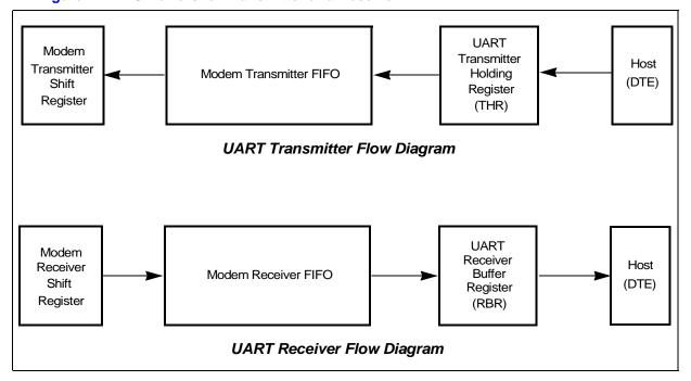
The register addresses are divided into two types: single-register access and multiple-register access. Most of the UART registers are single-register access (that is, only one internal register is accessible for a given register address). UART register addresses 3–7 are used to access a single internal register. The remainder of the UART register addresses (0–2) are used to access two or more internal registers.
