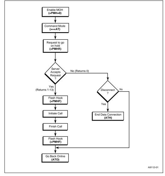
Figure 5. Modem-on-Hold: Initiating a Voice Call in Data Mode
