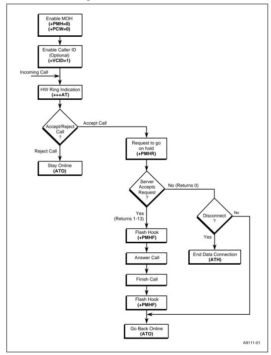
Figure 4. Modem-on-Hold: Incoming Voice Call in Data Mode
